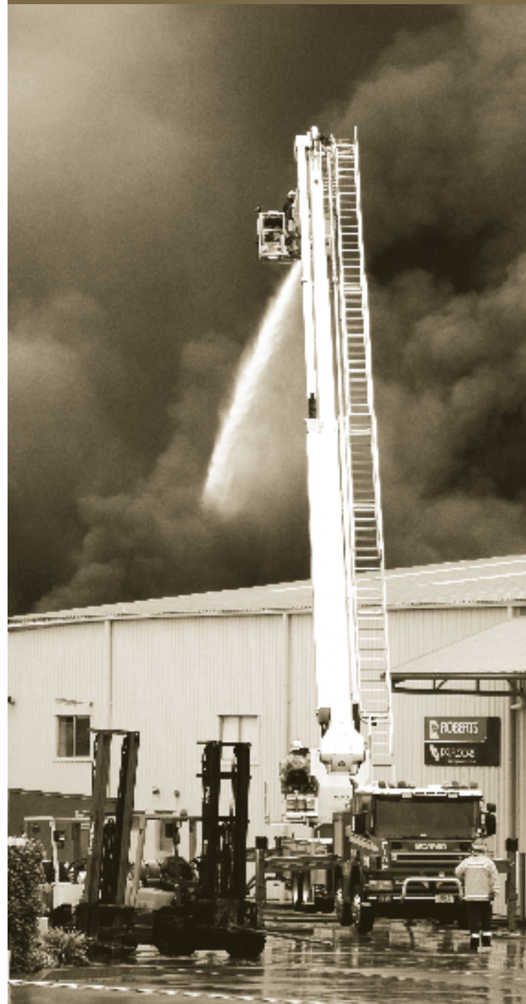
A QFRS turntable ladder platform allows crews to get above the flames at a factory fire.
